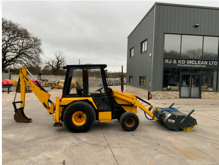
LEWIS BADGER WHEELED DIGGER
