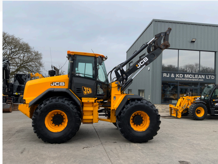
JCB 418S WHEELED LOADING SHOVEL (ST22214)
