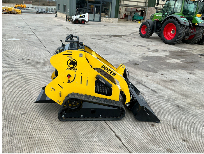
DOZER TRACKED SKID STEER LOADER (ST21558)
