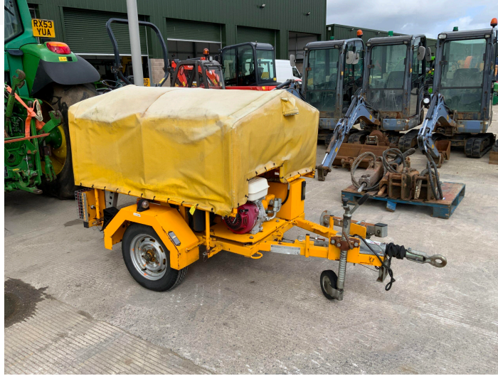
CBS 821 CABLE/ FIBRE OPTIC PULLING WINCH (ST18218)
