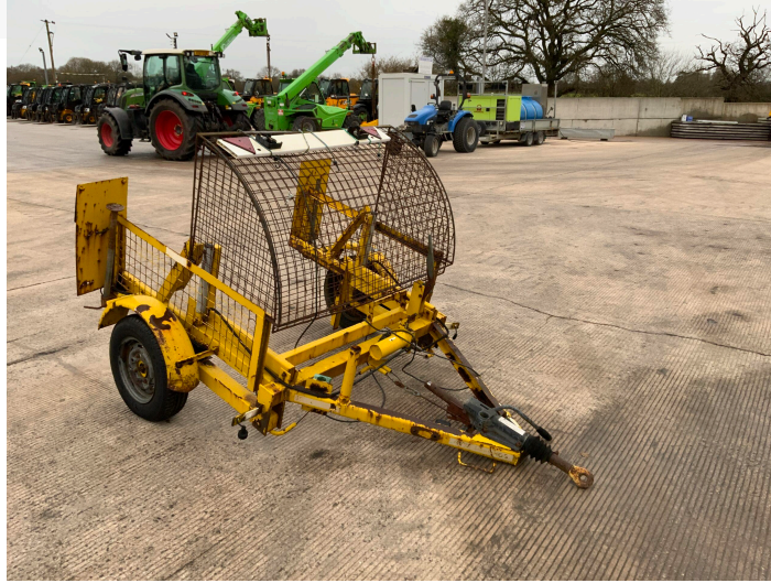
CABLE REEL TRAILER
