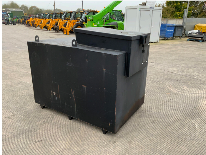
BUNDED DIESEL TANK
