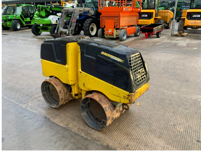
BOMAG BMP 8500 MULTI PURPOSE COMPACTOR ROLLER (ST20002)
