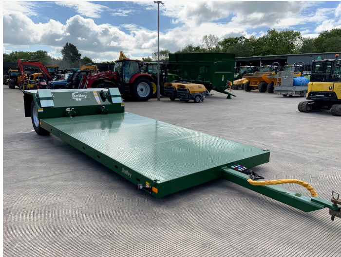
BAILEY 16FT 8 TONNE DROP DECK LOW LOADER
