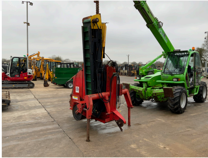
AFT WIZZ WHEEL TRENCHER
